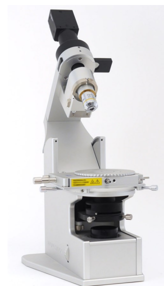
Linkam Imaging Station. Optics are tilted back to allow easy access to sample
